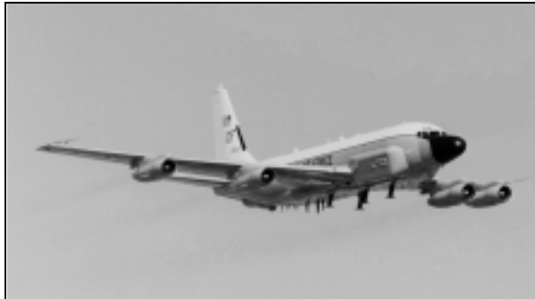
Figure 8. The Rivet Joint collection platform processes signal intercept data onboard the aircraft.
